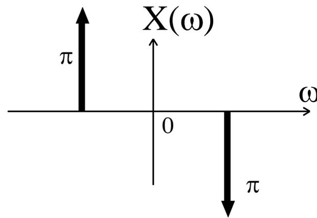
$$\sin \omega_0 t \longleftrightarrow j\pi [\delta(\omega + \omega_0) - \delta(\omega - \omega_0)]$$
