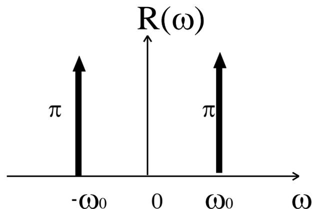
$$\cos \omega_0 t \longleftrightarrow \pi [\delta(\omega + \omega_0) + \delta(\omega - \omega_0)]$$
