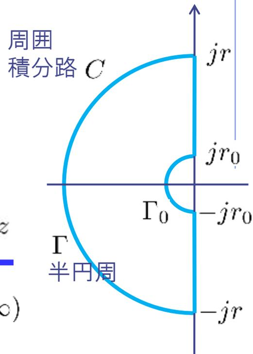
$$\int_{\Gamma_0} \frac{e^z}{z} dz = - \int_{\pi/2}^{3\pi/2} \frac{e^{r_0 \cos \theta + jr_0 \sin \theta}}{r_0 e^{j\theta}} \cdot jr_0 e^{j\theta} d\theta \quad \leftarrow z = r_0 e^{j\theta}$$
